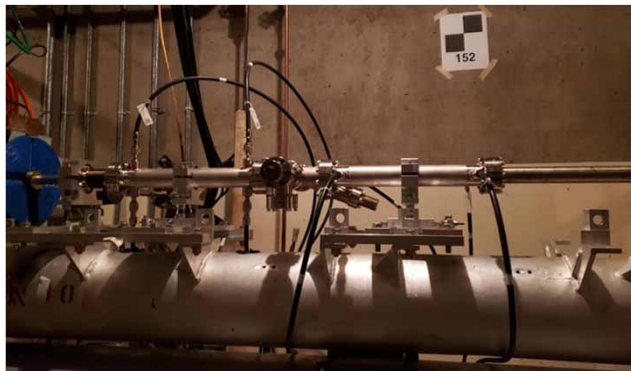
TEM striplines installed during winter 2021/2022
