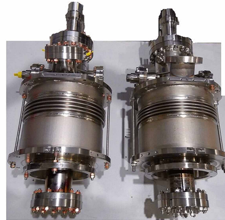
Cavities for operation with Cs 2 KsB photocathodes
