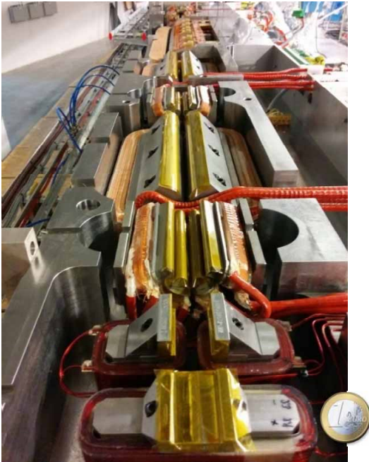
MAX IV 3 GeV: top view of a magnet block
