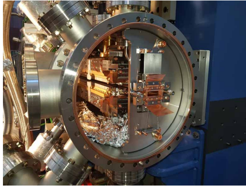
Movable gap of in-vacuum IDs can change between collimator and cavity
