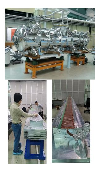
All components tested OK SCU cooldown is fine now SC coils need more work.
