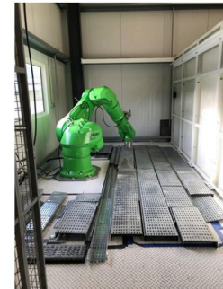
Robotized measurements done for the old SR components
