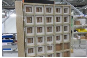
Magnet blocks ( \text{Sm}_2\text{CO}_{17} )
