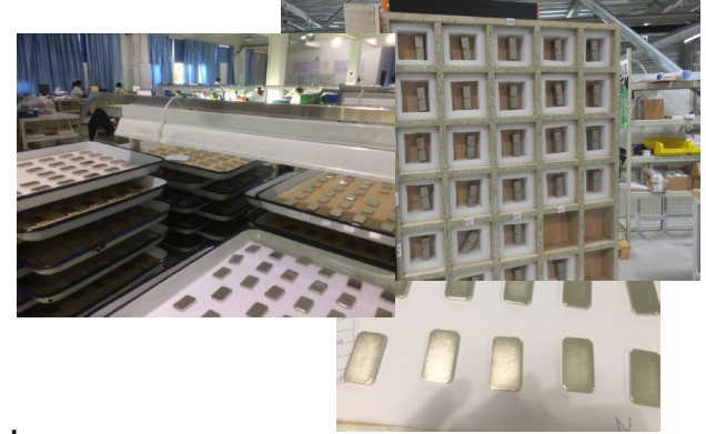
New magnet blocks before assembly
