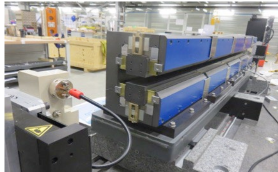
Magnetic measurements of full DL & final field tuning((stretched wire)
