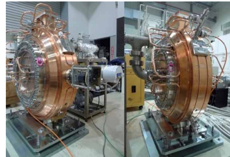
Figure 1: RF cavity with the compact HOM-damping structure.
