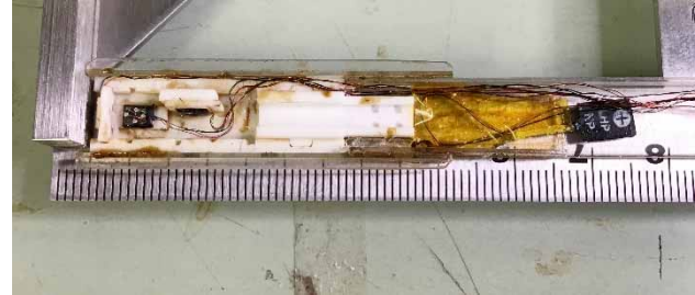
Figure 3: Photograph of a Hall sensor array, which can measure three-component magnetic fields along the z-axis. The second and fourth Hall sensors from the left are used to measure the B_{und} component.
