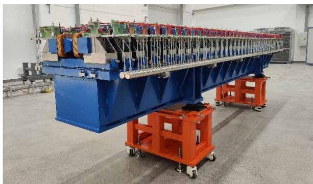
Figure 4: The THz undulator for SXFEL.
