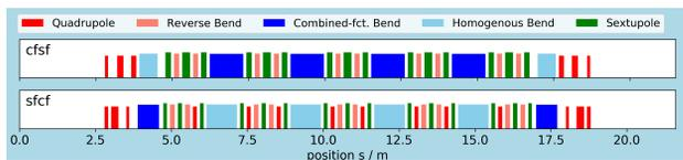
Figure 4: The lattices are named after the type of their bend in the UC and DSC. Top: cfsf (combined function, separate function) HOA-6MBA lattice. Bottom: sfcf HOA-6MBA.
