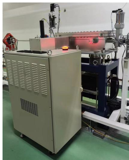
Figure 9: Kicker magnet and its high stability pulsed power supply installed in the undulator tunnel.
