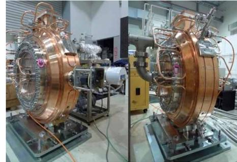
Figure 1: RF cavity with the compact HOM-damping structure.
