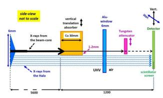
Figure 1: The main components and the paths of the X-rays of both the beam-core and that of the halo population.
