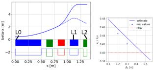
Figure 1: Left:  $\beta_r$  in half UC, regular (line) and for QD=0 (dashed line); magnet color code: MB: blue; RB: purple; QD: red, SF, SD: green. Right:  $v_x$ , analytic estimate (blue line), exact phase advance (stars), and option for HOA (red).
