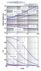
Figure 1: The estimated improvements from TPS to TPS-II on the relative brightness and CF. The red line represents the present operation conditions of TPS ( $\varepsilon_0 = 1.6 \text{ nm} \cdot \text{rad}$ , 500 mA). This calculation employs undulator with the same magnet length and period numbers, optics function of  $(\beta_x, \beta_y) = (5.353, 1.73) \text{ m}, \text{ and } \eta_x = 0 \text{ m}.$
