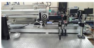
Figure 1: Laser Interferometer system on Hall probe bench.
