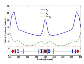
Figure 1b: Optical function with the help of gudrupole triplet to minimize the  $\beta_v$  at the core of each EPU.
