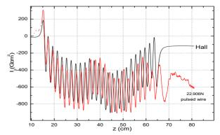
Figure 1: Second field integral at a wire tension.
