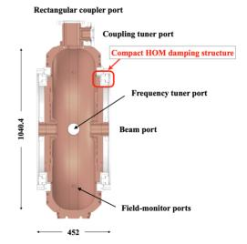
Figure 2: Cross-sectional view of the cavity.
