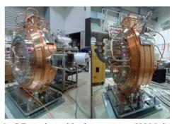
Figure 1: RF cavity with the compact HOM-damping structure.
