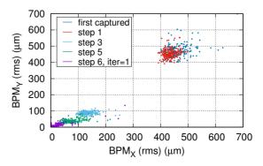
Figure 1: RMS BPM readouts at different steps.
