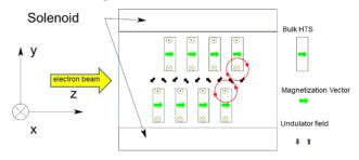
Figure 1: A schematic cross sectional view of a Bulk HTS SAU. When the magnetic field is changed by an external solenoid, a shielding current is induced inside the bulk HTS to cancel out the magnetic field change. The induced current produces a periodic alternating magnetic field along the z-axis.
