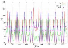
Figure 1: Optical functions of the double mini- $\beta_y$  lattice for 1/3 TPS storage ring.
