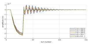
Figure 2: Orbit at the BPM number 1, which is inside the injection bump, during the ramp rise and after it goes off in about 1 turn. The oscillations are dumped quickly because of strong decoherence due to the high chromaticity.
