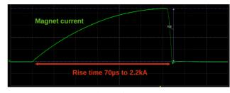
Figure 1: Pulse shape of the injection kickers.
