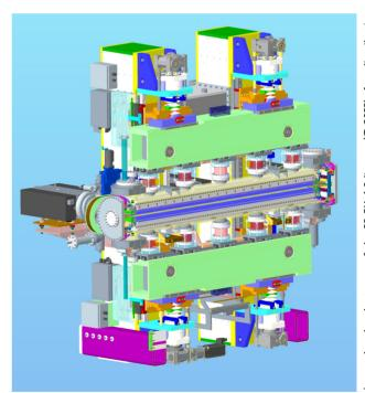
Figure 1: Model of CPMU-3 with the vacuum chamber cut away. The beams are light green with the bellows of the columns shown in red.
