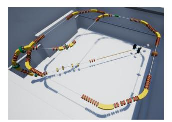
Figure 1: Artistic view of the cSTART project. The cSTART storage ring at a height of about 3.5 m is connected to the FLUTE injector by a complex 3D transfer line. The LPA (not shown) will be at the same height as the storage ring and uses the last part of the transfer line of FLUTE for injection.
