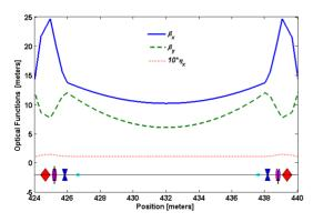
Figure 1a: Optical functions without the quadrupole tripole in the 12-meter-long straight.
