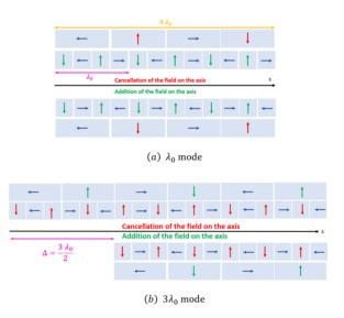
Figure 1: Configuration of magnet magnetization.
